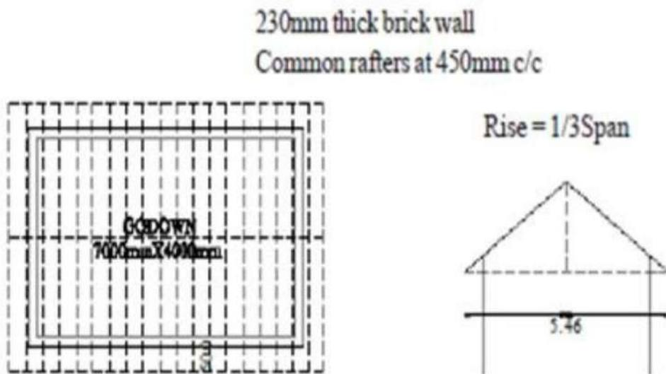
$$\text{a) Length of Common rafter} = \left(\frac{\text{length}}{2}\right)^2 + \left(\frac{\text{Span}}{3}\right)^2 = \sqrt{2.73^2 + \left(\frac{5.46}{3}\right)^2}$$
